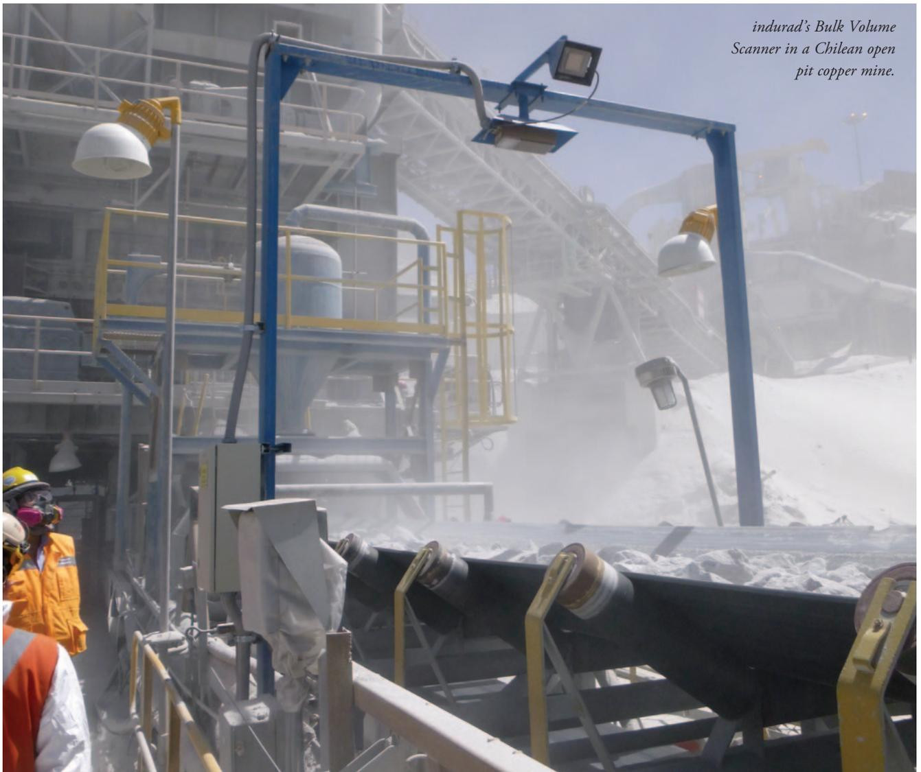
*indurad's Bulk Volume Scanner in a Chilean open pit copper mine.*
