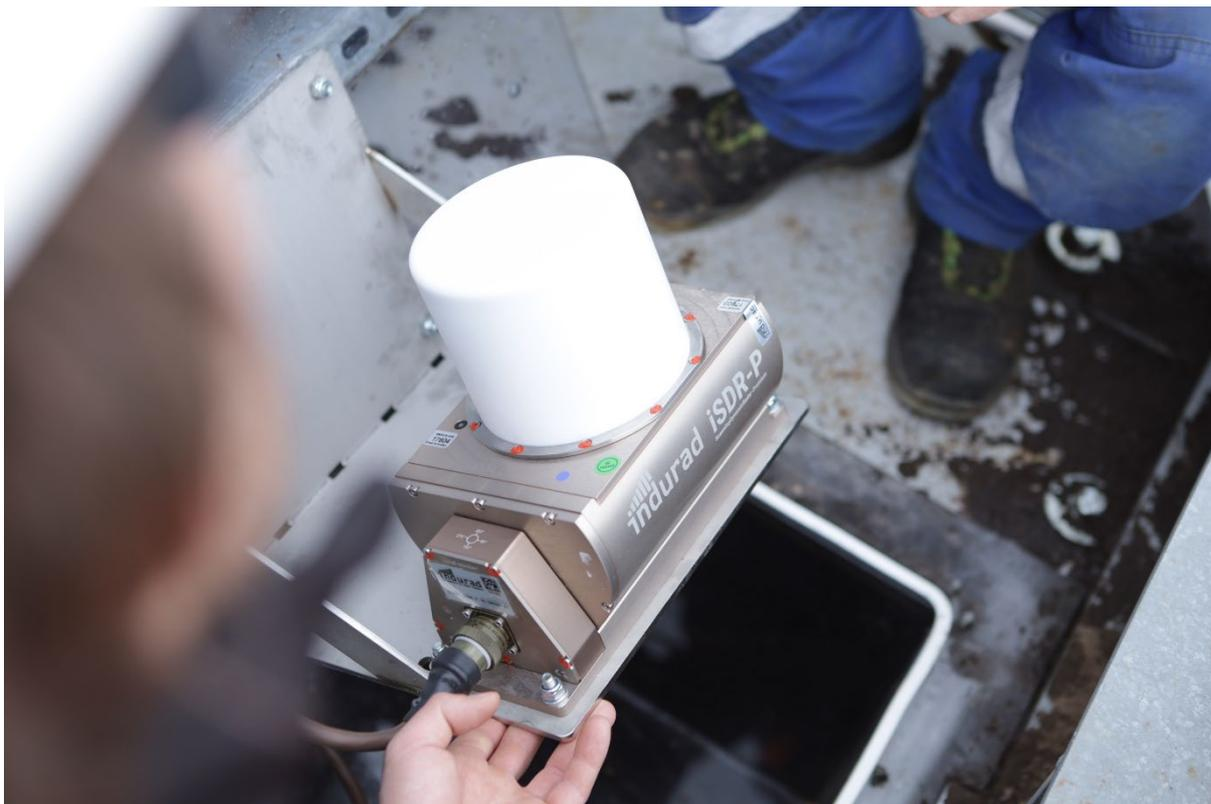
Picture (2): iSDR-P: Robust 3D radar built for harsh and dusty environment
