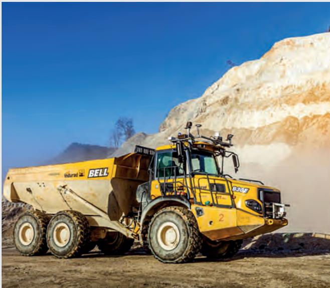
*indurad has successfully demonstrated that trackless mobile machine automation in harsh mining environments including terrestrial mapping is feasible with radar-only perception*
